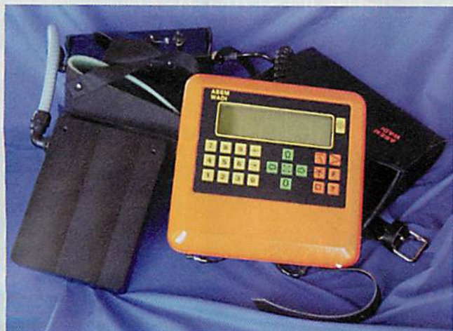
OLD INNOVATION A retired engineer uses an out-of-production device to read very-low-frequency radio waves to find water trapped in underground rock.
